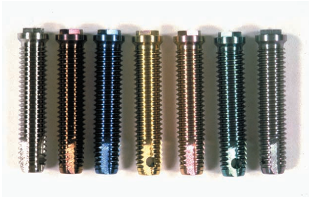
Fig. 3. Colouring of the clinical titanium implants prepared by galvanostatic oxidation; the native oxide film (reference colour) of a clinical screw implant to the left, the interference colours consecutively anodized at 20, 40, 80, 100, 180 and 200 V to the right, in 0.5 M tartaric acid.
